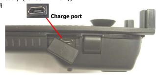
DC9272N is with Li-Ion battery inside. When in charging, please use the original power adaptor of OTG device (recommend). Through it, it charges both OTG device and DC9272N internal battery at the same time. When in low battery (Red LED flashing), please charge it immediately.
